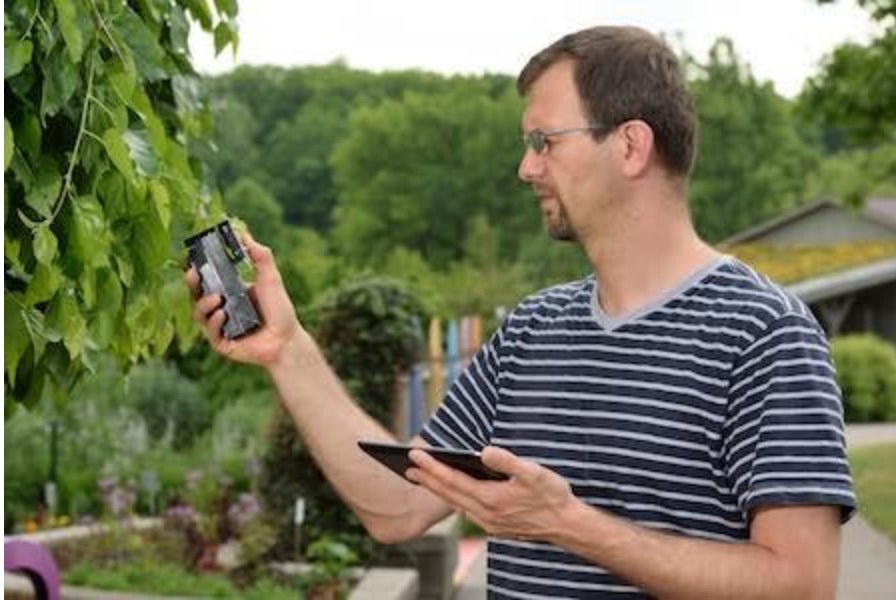
Figure 3 PhotosynQ in action: the device collects data. A mobile app uploads it to an online platform for further analysis. By Harley J Seeley Photography
