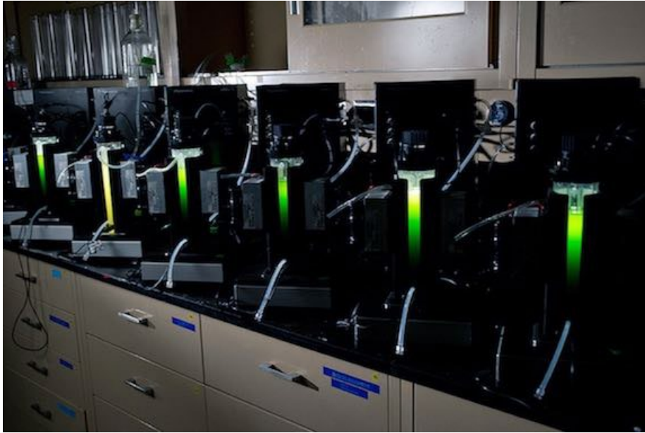
Figure 2 Algae were stress tested in these bioreactors made in the Kramer lab. Each is a 'pond in a jar' that can reproduce real-world settings for testing purposes. By G.L. Kohuth
